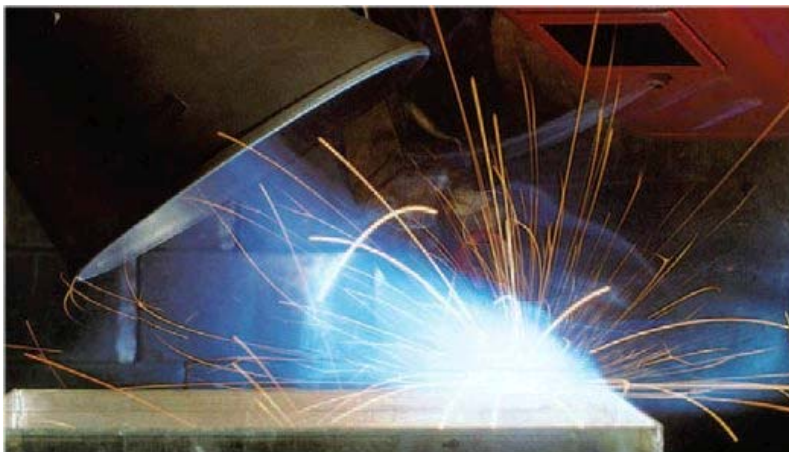
Figure 1 - Proper positioning of fume Exhaust Hoods (left-right)
