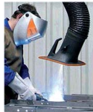
Figure 1 - Proper positioning of fume Exhaust Hoods (left-right)
