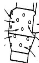
Figure 23 – Flared annular sleeve with holes
