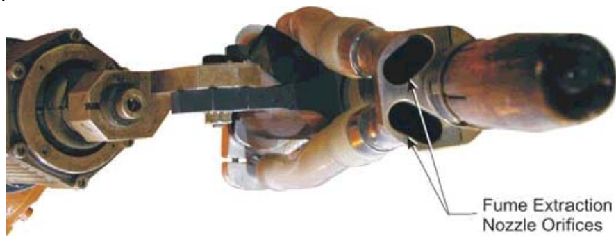
Figure 55 – Fume exhaust torches for robotic applications. Photo courtesy of Rimrock-Wolf Robotics Inc. – USA (upper) and Aspirmig Srl – Italy (lower)
